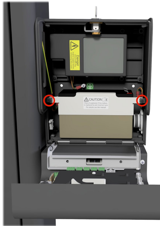
Figure 21 - Location of fixing screws on the battery bracket
