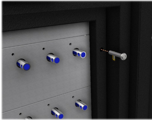
Figure 37 – Removing Pin Screws from the Receptor Frame
