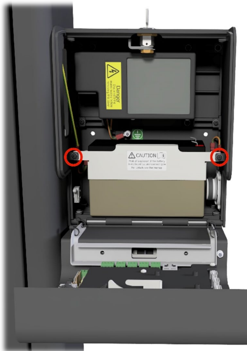
Figure 45 - Location of fixing screws on the battery bracket
