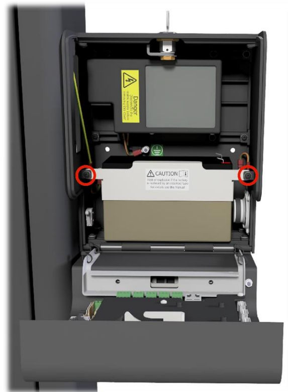
Figure 42 - Location of fixing screws on the battery bracket
