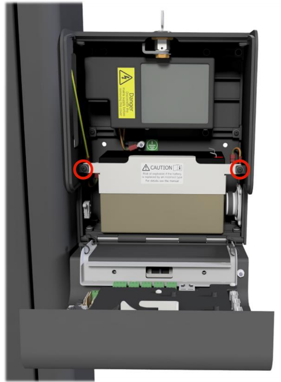
Figure 21 - Location of fixing screws on the battery bracket
