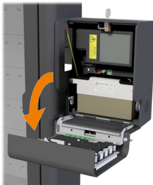
Figure 20 – Pulling down the Control Panel to reveal the battery
