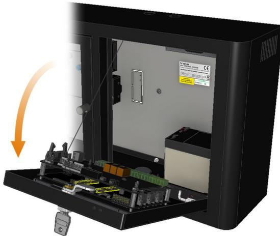
3. To release the door you will need to locate the lock mechanism and lift the lock catch up.
