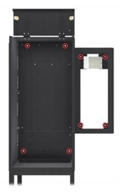
4. Once securely fixed to the wall the mains and communications cables need to be run to the unit. 20mm knockout holes are provided in the top and bottom of the pod. The power supply and communication cables should be brought to the top or the bottom of the Pod via 20mm trunking.
