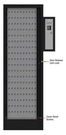
5. Using a 4mm Allen Key, remove the Cover Panel Screws one at a time and remove the cover panels.
