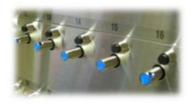
**NOTE:** Once a user pushes a receptor button the system will check if the user has the correct <u>access level</u> to remove the iFob. If they do not possess the correct access levels, the system will deny the removal of the iFob.
