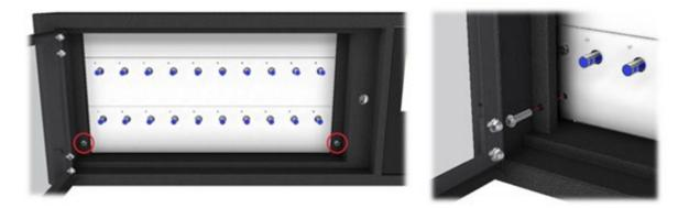
7. Using a large flat bladed screwdriver, remove the screws from the receptor strip you wish to release the iFobs from. Remove the strip, carefully disconnecting the receptor ribbon cable.
