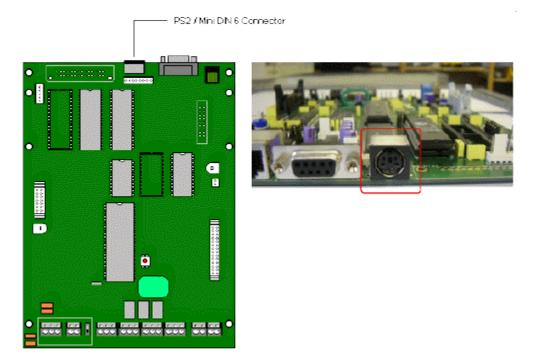
2. A **PS2 to Terminal Block Interface Cable** is required allowing termination of the fire alarm switch or break glass switch. The cable can be supplied upon request. See below for a diagram showing the connections required:
