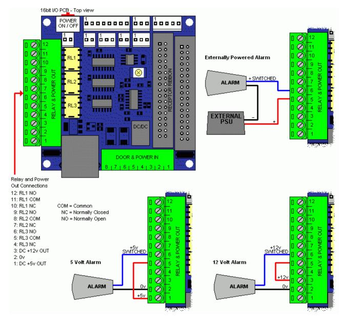
**NOTE:** At no point should mains be wired into the Alarm Relay Output.
