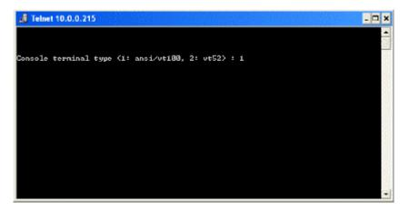
Please note, if the following text "Console terminal type (1: ansi/vt100, 2: vt52) : 1" does not appear on the screen then check the default IP Address is within range of the IP Address that you are running telnet from. The default subnet mask of the TMED is 255.255.255.0 with no gateway.
