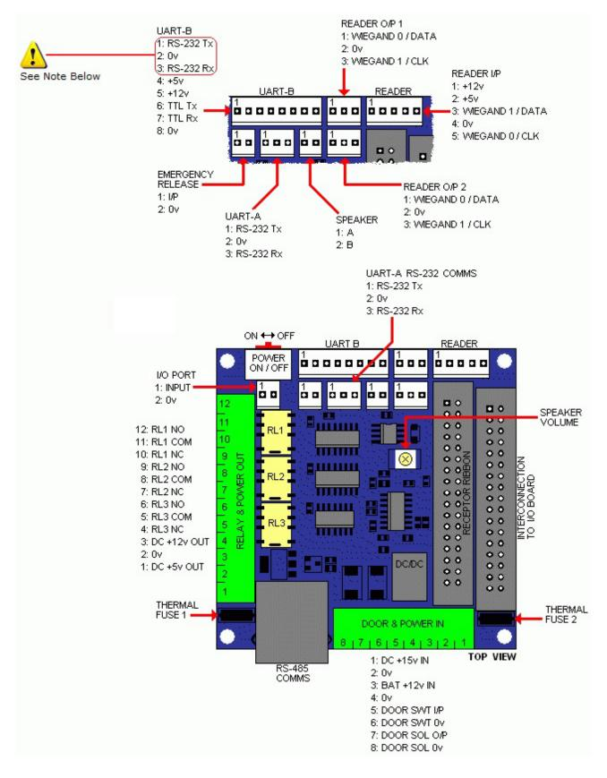
**NOTE:** Version 1.3.0 UART-B pins 1 and 2 (RS-232 TX and 0v) have been switched (compared with Version 1.2.0) so as the same RS232 cable can now be used for UARTA *and* UARTB.
