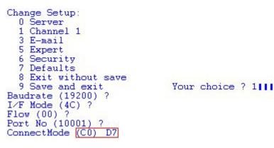
The 'Connect Mode' will be set up as C0 and needs to be changed to D7. Simply enter D7 and select Enter.
