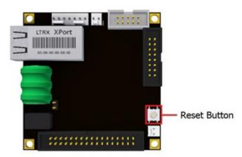
b. Keeping hold the '#' key, release the Reset Button and the following message will appear...
