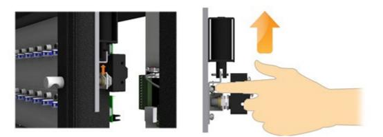
5. Undo the plastic Wing Bolt then close and lock the Control Panel. You will now be able to swing open the Control Panel Door.
