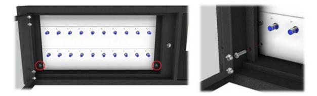
7. Using a large flat bladed screwdriver, carefully remove the blanking strip at the top and remove the two receptor strips and carefully disconnect the receptor ribbon cable. Put the receptor strips in a safe place until needed, noting where they came from as they must be returned to the same location.
