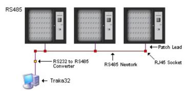
It is recommended that you install the RJ45 Wall ports behind the Traka Control Panels to prevent anyone from tampering with the connections. The Cat 5 cable should not span more than 500 metres in length and should not run alongside power cables.
