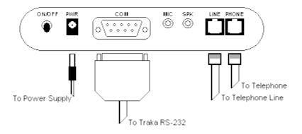
5. Fit the modem behind the Control Panel of the Traka system, feeding the Modem Telephone Lead out through any of the cable knockout holes on the Pod/cabinet and connect to an Approved British Telecom Telephone Socket.
