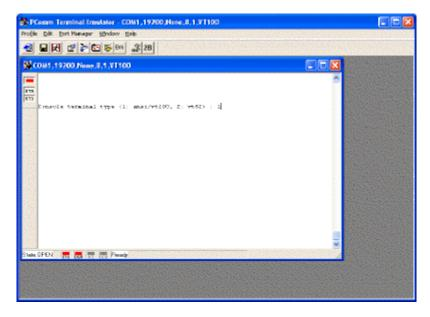
Please note, if the following text "Console terminal type (1: ansi/vt100, 2: vt52) : 1" does not appear on the screen then try powering down the TMED, waiting 5 seconds and powering back up again.
