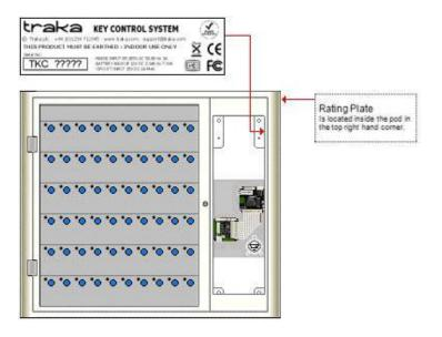
For Traka Products such as the **L-Series, Lockers and Access control Pods**, the Rating Plate is located inside the Pod. You will need to remove the control panel in order to view the Rating Plate. Additionally there will be another label on the outside of the Pod on the right hand side stating were you can find the Rating Plate.
