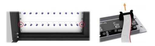
7. Using a small flat blade screwdriver, you will be able to pull back the small solenoid blade that holds the iFob in place and remove the iFob.
