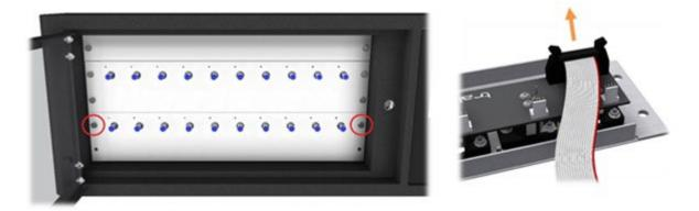
8. Using a small flat blade screwdriver, you will be able to pull back the small solenoid blade that holds the iFob in place and remove the iFob.
