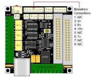
8bit Control PCB - Top view
