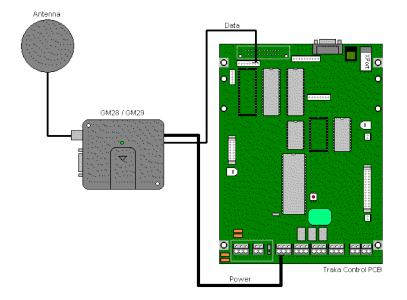
**NOTE:** To integrate the Sony Ericsson GM28 or GM29 module with the Traka Control PCB v2.30.04, the following modifications are required:
