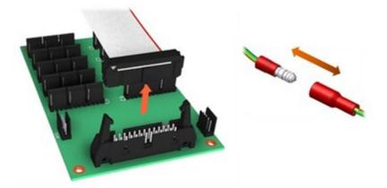
4. Depending on your system configuration it's possible that lock cables and RFID cables from adjacent modules may also be connected to the PCB. If this is the case then these cables must also be disconnected to allow the module to be freely removed.
