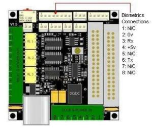
Biometrics Connections 1: 0v 2: Tx 3: Rx 4: +5v 5: N/C 6: N/C 7: N/C 8: N/C 1: 0v
