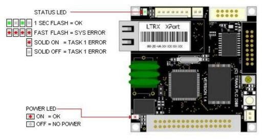
5. NOTE: The status LED should flash when there is an application loaded and is running. If there is no application loaded, then the status LED will be on solid and the LCD will show:
