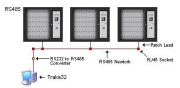
It is recommended that you install the RJ45 Wall ports behind the Traka Control Panels to prevent anyone from tampering with the connections. The Cat 5 cable should not span more than 500 metres in length and should not run alongside power cables.
