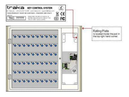
For Traka Products such as the **L-Series, Lockers and Access control Pods**, the Rating Plate is located inside the Pod. You will need to remove the control panel in order to view the Rating Plate. Additionally there will be another label on the outside of the Pod on the right hand side stating were you can find the Rating Plate.
