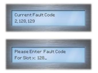
If you wish to clear this fault, press the \* (star) key to delete the fault code and then press the # (hash) key. If you do not wish to clear the fault, simply press the # (hash) key without deleting the number to keep the fault.
