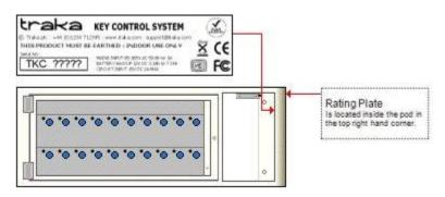
For the Traka **S-Series** the Rating Plate is located on the inside, you will need to remove the control panel in order to view the Rating Plate. Additionally there will be another label on the outside of the S-Series on the right hand side stating were you can find the Rating Plate.
