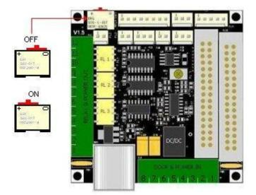
4. Check that Power LED comes on and after a short while that the Status LED starts to flash.
