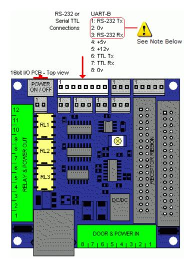
**NOTE:** Version 1.3.0 UART-B pins 1 and 2 (RS-232 TX and 0v) have been switched (compared with Version 1.2.0) so as the same RS232 cable can now be used for UARTA *and* UARTB.
