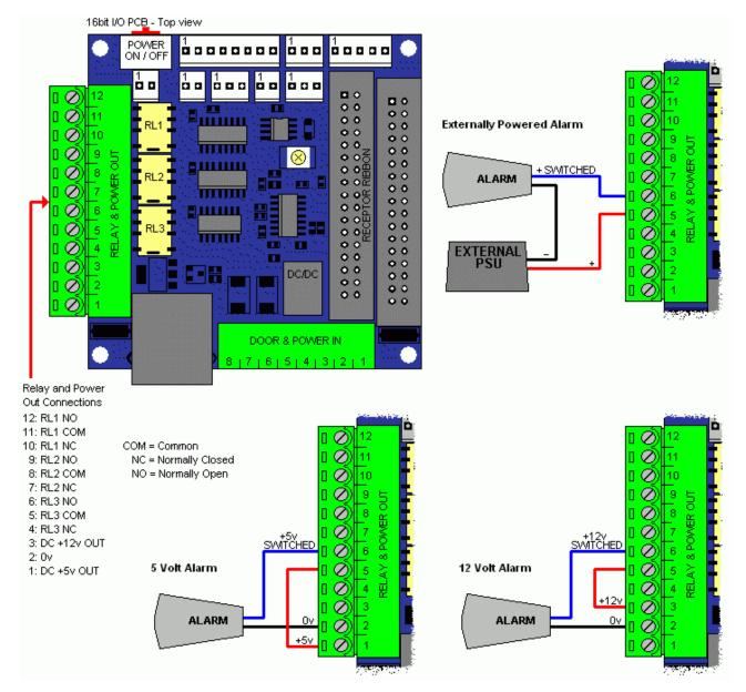
**NOTE:** At no point should mains be wired into the Alarm Relay Output.
