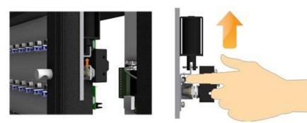
4. Undo the plastic **Wing Bolt** then close and lock the Control Panel. You will now be able to swing **open the Control Panel Door**.
