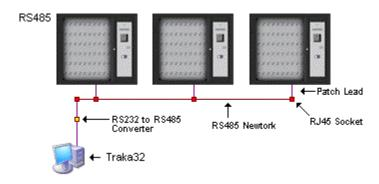
It is also possible to combine the RS485 communications with Ethernet to allow a single Traka32 client to administer the Traka Systems and as many additional 'view only' Traka32 clients as is required.
