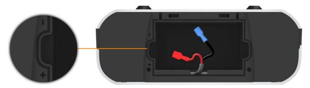
4. Connect the battery to the battery cable. Use the connection code in the section above for guidance.
